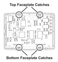
3. Using fingers or a screwdriver, pry the top set of faceplate catches loose and PUSH the faceplate forward slightly.
