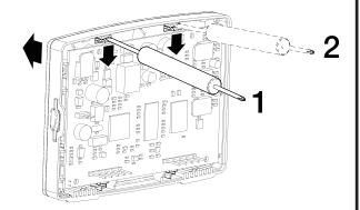
4. After the top set of catches are loose, pry the bottom set of catches loose and PUSH the faceplate forward to detatch it from the front housing.
