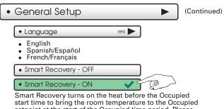
start time to Bring the room temperature to the Occupied setpoint at the start of the Occupied time period. Please allow 4-8 days for Smart Recovery time to adjust. When used with a heat pump, electric strip heat will be disabled while Smart Recovery is active.
