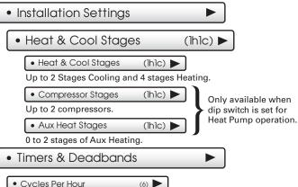
At 6 cycles per hour, the HVAC unit will only be allowed to energize once every 10 minutes. The Cycles Per Hour limit may be overridden and reset by pressing the WARMER or COOLER buttons.
