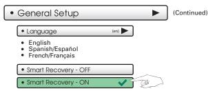
Smart Recovery turns on the heat before the Morning start time to bring the room temperature to the Morning setpoint at the start of the Morning time period. Please allow 4-8 days for Smart Recovery time to adjust. When used with a heat pump, electric strip heat will be disabled while Smart Recovery is active.
