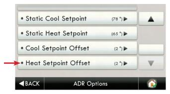
The user may adjust the ADR Heat offset. During an ADR event the heating setpoint will be adjusted by the amount of degrees configured in this step.
