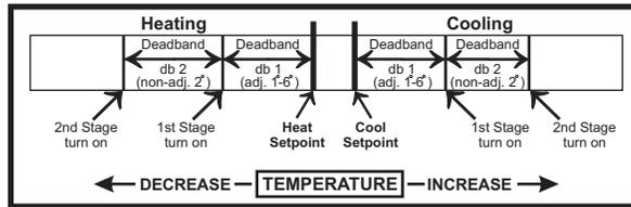
The above figure assumes the minimum on time for the prior stage has been met to allow the next stage to turn on, once the deadbands have been exceeded.
