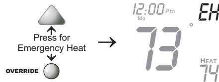
**Operation** - During Emergency Heat operation the thermostat will turn on the fan and the 2nd stage of heat when there is a demand for heat. Also during Emergency Heat, the 1st stage of heating or cooling will be unavailable.
