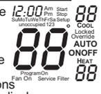
**3** Press the MODE button once. The thermostat temperature will be displayed and may be calibrated using the UP or DOWN buttons.
