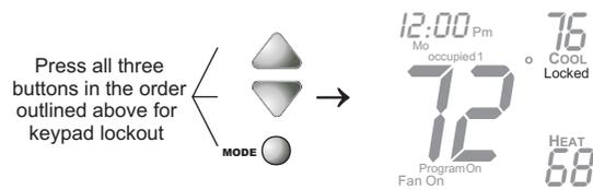
To **unlock** the keypad, press and hold the MODE button. While holding the MODE button, press the UP and DOWN buttons together. The LOCKED icon will disappear from the display, then release the buttons.
