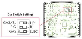
\*Reversing valve choice, 0 or B, is dependant on the type of valve installed in the heat pump.
