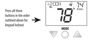
To **unlock** the keypad, press and hold the MODE button. While holding the MODE button, press the WARMER and COOLER buttons together, for two seconds.
