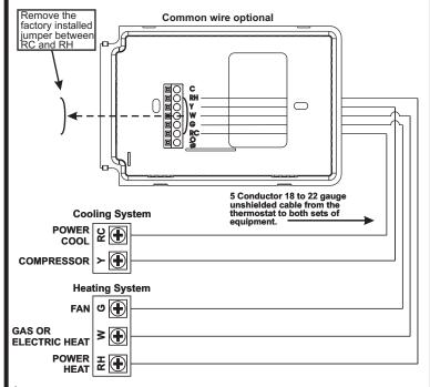
\* If a common wire is used it must be connected to the furnace common terminal. If a common wire is not used the thermostat must be powered by two AA alkaline batteries. These batteries must be replaced (page 6) each year or when the Low Battery indicator is displayed (page 3).
