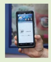
Using Venstar's Skyport® Cloud Services, the temperature information from the ColorTouch thermostats and Venstar Remote Sensors can be remotely monitored using the Skyport interface on a computer or by using the free Skyport Mobile App. Important email alerts are automatically sent to Queirolo's and the Baskin Robbins store owner when temperatures go above pre-determined safe temperature settings.
